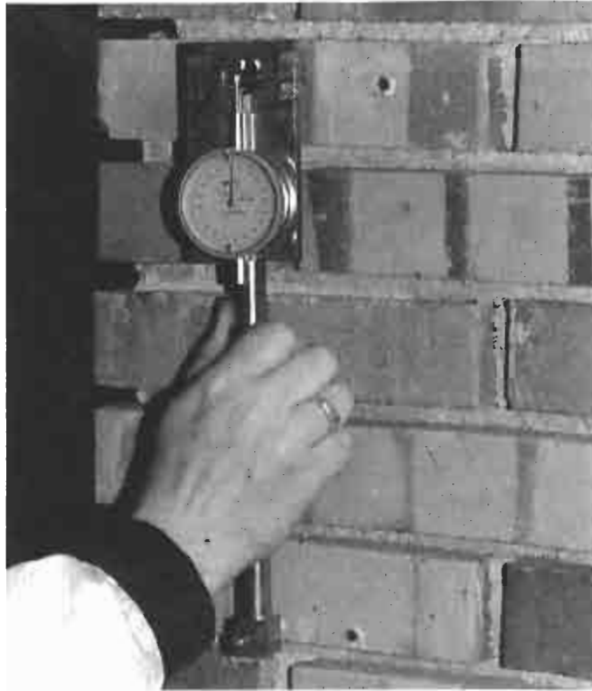
Photo 1 Removable mechanical deformometer used in common practice.
