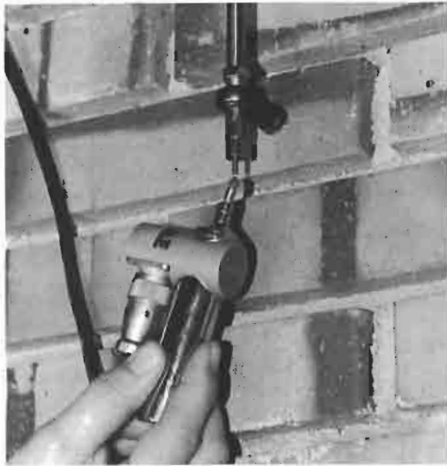
Photo 3 Displacement sensor device: detail of an anchorage
