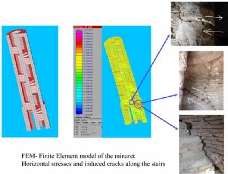
FEM- Finite Element model of the minaret
