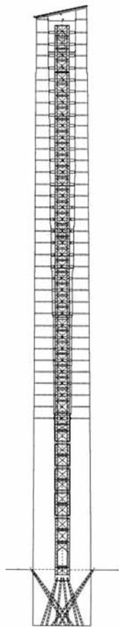
The dead load of the masonry is partially transferred to the inner tower by means of about 300 prestressed **sub-vertical cables**, laying in the interstice between the masonry and the steel tower. The new structure takes into account the culture of preservation, such as adoption of strengthening work which stands
