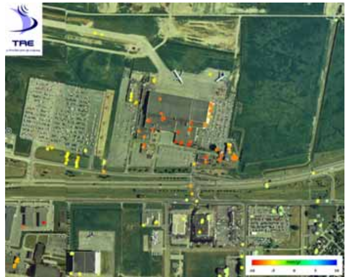
Figure 8b. The Air Canada hangar at Vancouver International Airport. The land surrounding the hangar is settling at approximately half the rate of the building, itself.
