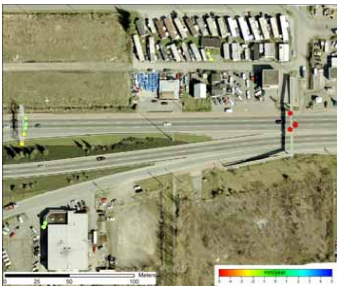
Figure 8a. PS identified on a traffic direction gantry and on a pedestrian footbridge in the alluvial sediments within the City of Surrey.
