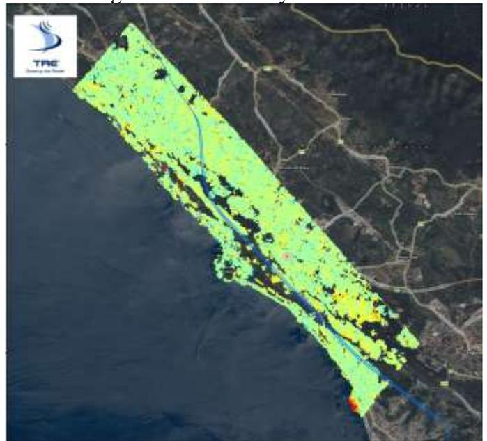
Figure 2. Project phase: PSInSAR™ analysis over the new Venice-Trieste railway line (preliminary design).
