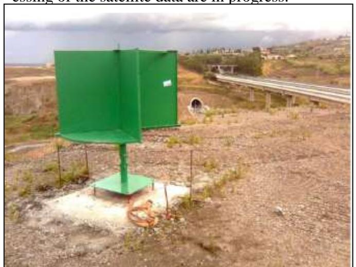
Figure 7. Monitoring phase: View of an artificial reflector installed on the slope of Tracocchia, Sicily.
