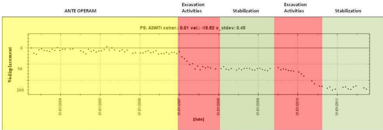
Figure 5. Displacement historic time series representing the effects induced by tunnel excavation.
