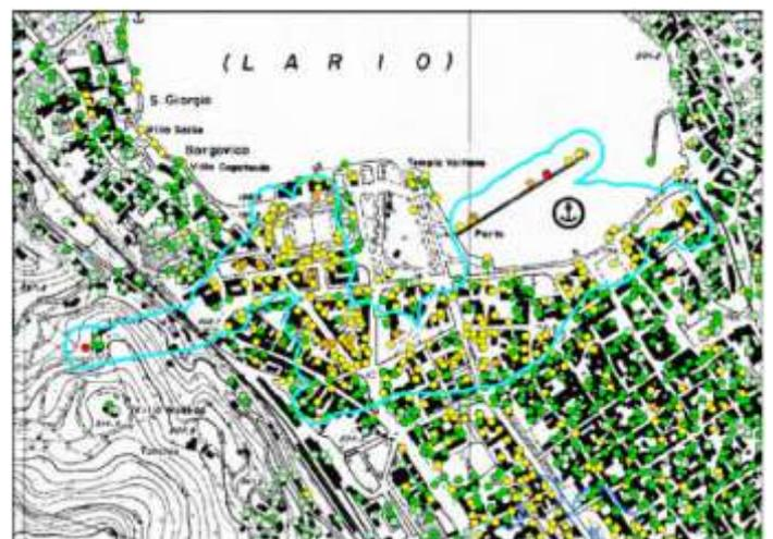
Figure 13. Como lake. SqueeSAR™ analysis performed over the area exposed to hydro-geological risk.
