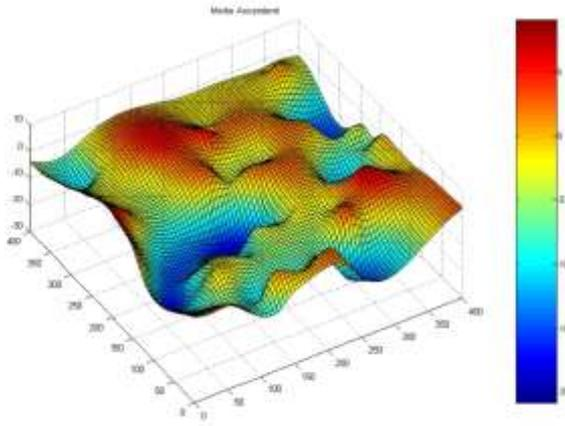
Figure 11. Settlement [mm] represented in a 3D surface diagram
