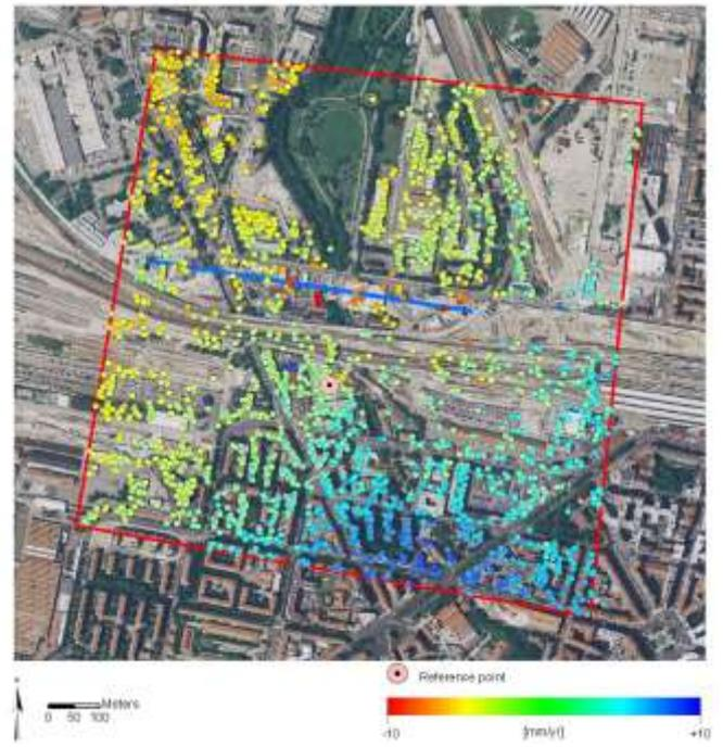
Figure 4. Construction phase: PSInSAR™ analysis over Bologna. PS/DS Average Velocity [mm/yr] along satellite line of sight.
