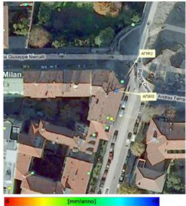
Figure 13. PSInSAR™ analysis over Milan. Time range 2003-2009. PS/DS Average velocity [mm/yr] along satellite line of sight
