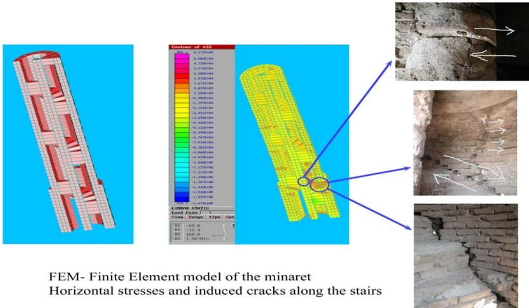
FEM- Finite Element model of the minaret
