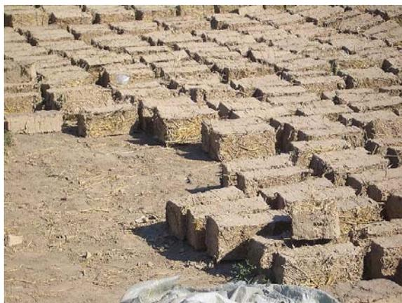
Figure 1: adobe bricks during drying process
